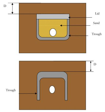
Figure 6C: Explanation of the Depth of the Direct Burial System
