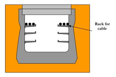
Figure 6B: Example of Draw-in Culvert System
