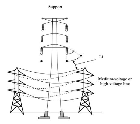
Figure 10: Proximity and Crossing with Medium-voltage Lines and High-voltage Lines
