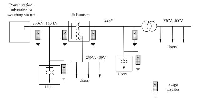
Figure 11: Installation Points for Surge Arresters
